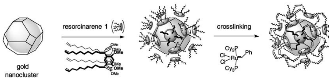
FIGURE 1 Schematic of nanocluster encapsulation by resorcinarene 1 , followed by engagement via olefin metathesis.
